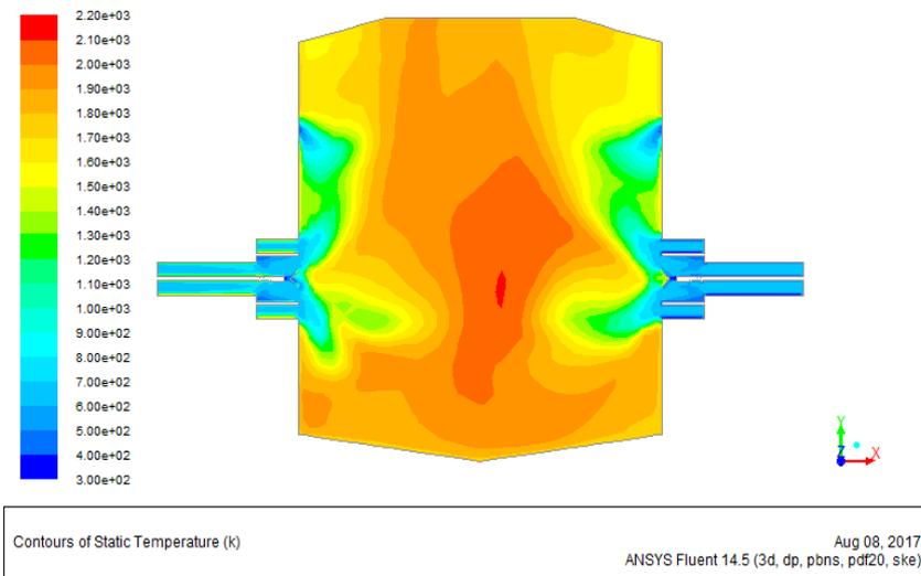
Figure 1 - The calculated field of the temperatures (K) in vertical section of the furnace along the axes of the 2-nd and 5-th burners (above), as well as in horizontal sections at level of the burners axes and in the cross section of the overpressure (below).
